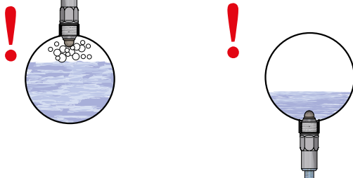
Fig. 7: Installing the sensor in the pipe
